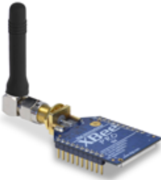
Transceiver used to send and receive RF signals. [4]
